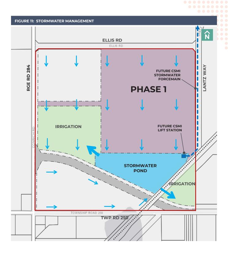
Road ROW cross sections with associated collection and conveyance systems will be developed within the Industrial portions of the Plan area to augment and support the proposed stormwater management system. Surface drainage from each lot will be collected and conveyed to the stormwater ponds.
